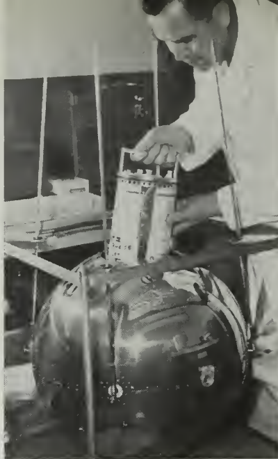
IGY SATELLITE program included Navy's development of Vanguard rocket and satellites. Here, Vanguard is readied and instruments are inserted.
